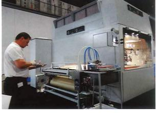
the guns from the reciprocating arm in few seconds and plug in a new set ready to use. The previous set of guns can also be flushed while the machine is spraying another colour. This system also reduces paint waste between colour changes.
