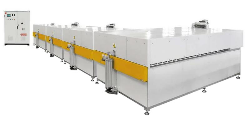
The working width can vary from 600mm to 3,300mm.
